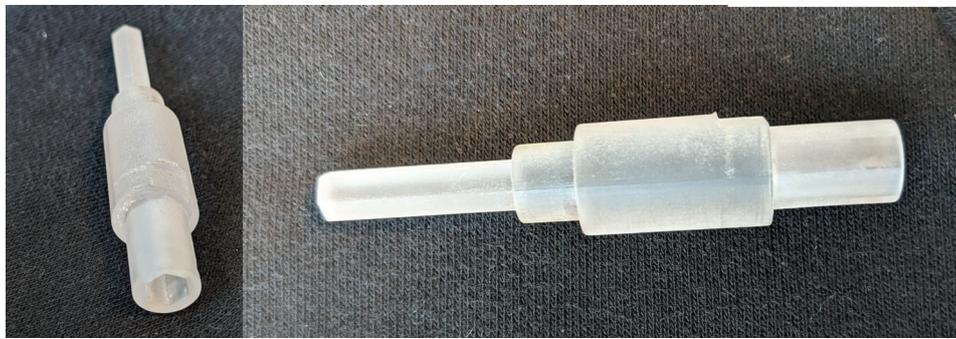
**Figure 5.8** The final shaft design, printed in plastic seen from two angles
