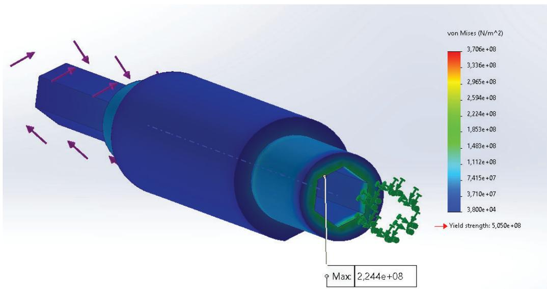
**Figure C.2** Simulated stress results on the encoder shaft due to manual drive of the motor shown at a different angle
