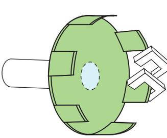
A green circular disk with a central hole and several radial slots is mounted on a white shaft. A white forked wheel is attached to the outer edge of the disk. A small rectangular sensor assembly is positioned to the right, with red dashed lines indicating the optical path through the slots of the wheel. | Optical encoder with a forked wheel, glued on motor shaft end                       |
