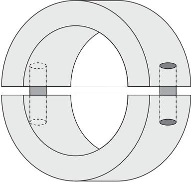
A 3D perspective drawing of a linear clamp or two-piece shaft collar. It consists of two separate, thick, semi-circular pieces that meet at a central point. A cylindrical shaft is shown passing through the gap between the two pieces, with shaded sections indicating the contact points on both sides. | <p>Linear clamp/two piece shaft collar - Available solution clamping around the shaft, may have trouble centering the motor shaft.</p>                                            |
