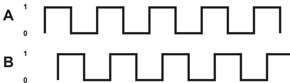
**Figure 2.1** The signal output from two optical sensors A & B from rotating a forked disc intermittently blocking them. 1 means the sensor is blocked and 0 means it is not blocked.
