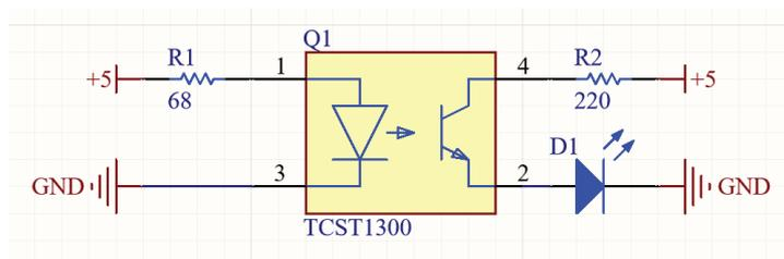
**Figure 5.6** Test circuit for optical encoder
