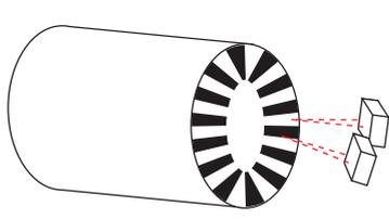
A cylindrical motor housing is shown in perspective. The end face features a circular disk with alternating black and white radial segments. A small rectangular sensor assembly is positioned to the right, with two red dashed lines indicating the optical path from the sensor to the disk's surface.           | Optical encoder with reflective tape on motor shaft end                             |
