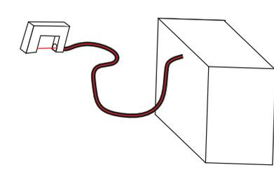
A small rectangular sensor assembly is on the left. A red fiber-optic cable connects it to a larger rectangular box on the right. The cable enters the box from the top and exits from the bottom, suggesting an internal measurement point.                                                                       | Optical encoder with fiber-optic cable to have measurements in a different location |
