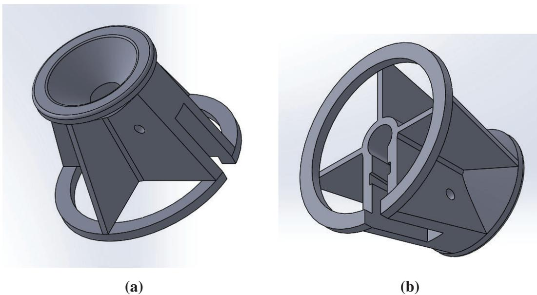
**Figure 4.2** The attachment for holding the micro-switch in place to detect any objects entering the encoder seen from the top (a) and bottom (b)
