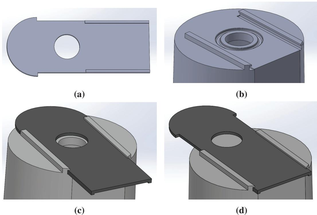
**Figure 5.16** CAD models of the lid for safety stop and sealing. Both the separate parts; the lid (a) and the housing with rails (b) as well as the parts assembled in the open (c) and the closed position (d) are shown.
