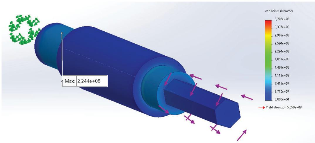
**Figure C.1** Simulated stress results on the encoder shaft due to manual drive of the motor
