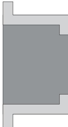
**Figure 4.5** A plain bearing design that allows for a shaft to be inserted all the way as to ascertain the exact position of the shaft in relation to the housing where the bearing is attached
