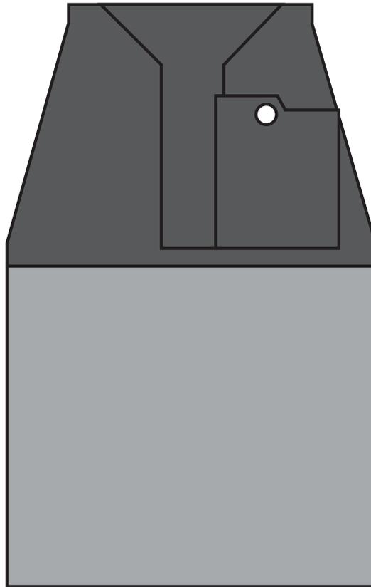
**Figure 4.4** A schematic assembly of the micro switch holder (dark grey) attached to the end of the encoder housing (light gray)
