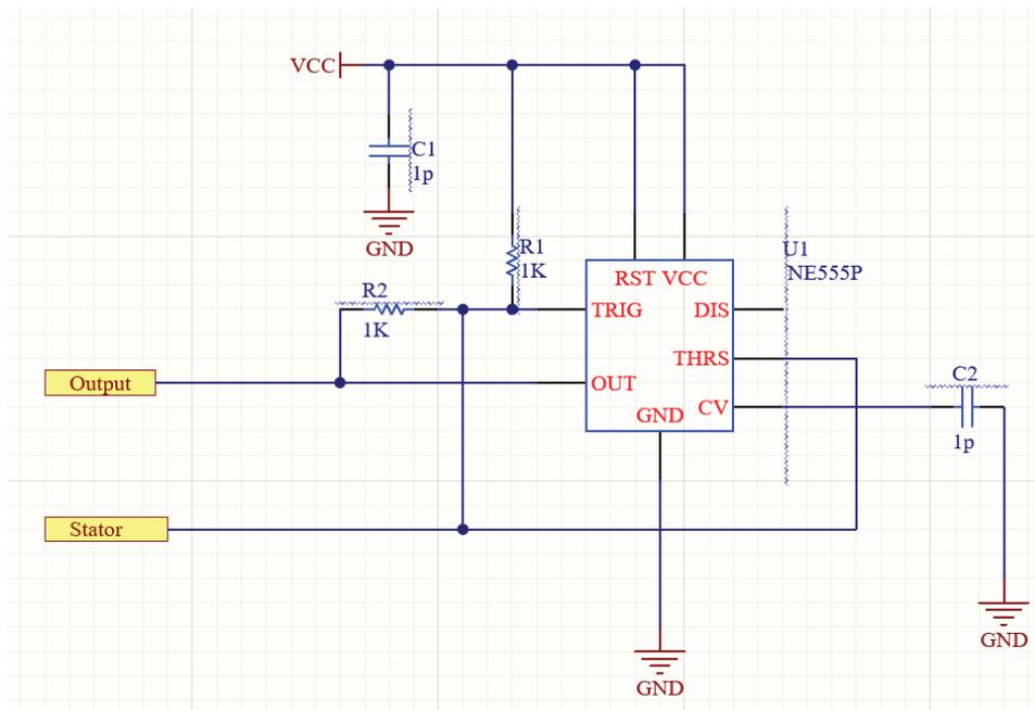
**Figure 5.3** Test circuit for capacitive encoder
