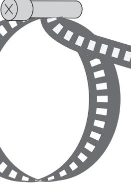
A 3D perspective drawing of a hose clamp. It features a dark, flexible, ring-shaped band with a series of rectangular slots along its length. A cylindrical shaft is shown passing through the ring, with a small circular fastener (a bolt with a cross) visible at the top where the band is clamped.      | <p>Hose clamp - A readily available solution to clamp the motor shaft. May have troubles clamping and centering a wide array of motor shaft diameters.</p>                        |
