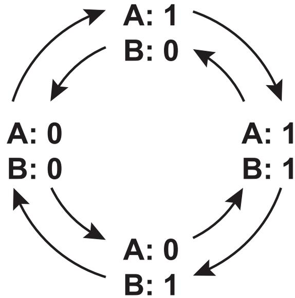
**Figure 2.2** The rotation derived from two optical sensors A & B being blocked and unblocked by a forked wheel
