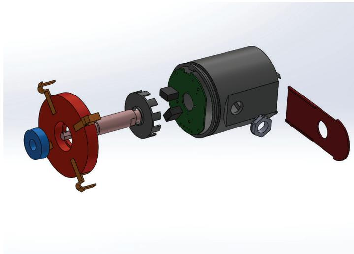
**Figure 7.2** Exploded view of the encoder CAD model
