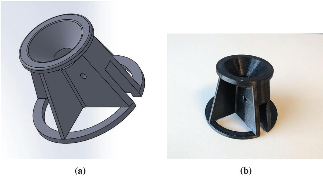
**Figure 5.14** CAD model (a) and physical prototype (b) of the micro-switch holder and crank guide for shaft detection
