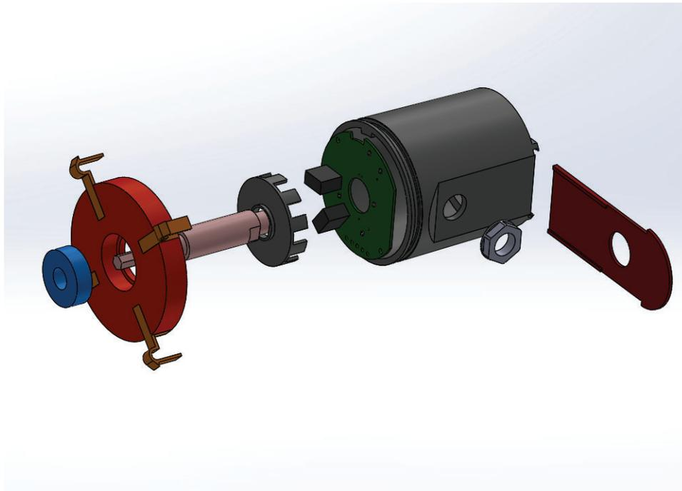
**Figure 6.1** Exploded view of the encoder CAD model
