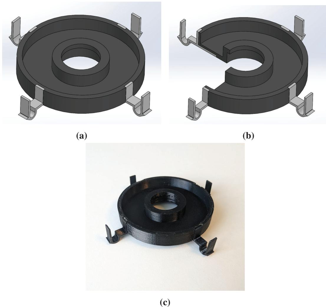
**Figure 5.12** The assembled base plate with snap-on connectors, two CAD models (a) & (b) with one having a quarter hidden to display the snap-on mount position as well as the physical model (c)
