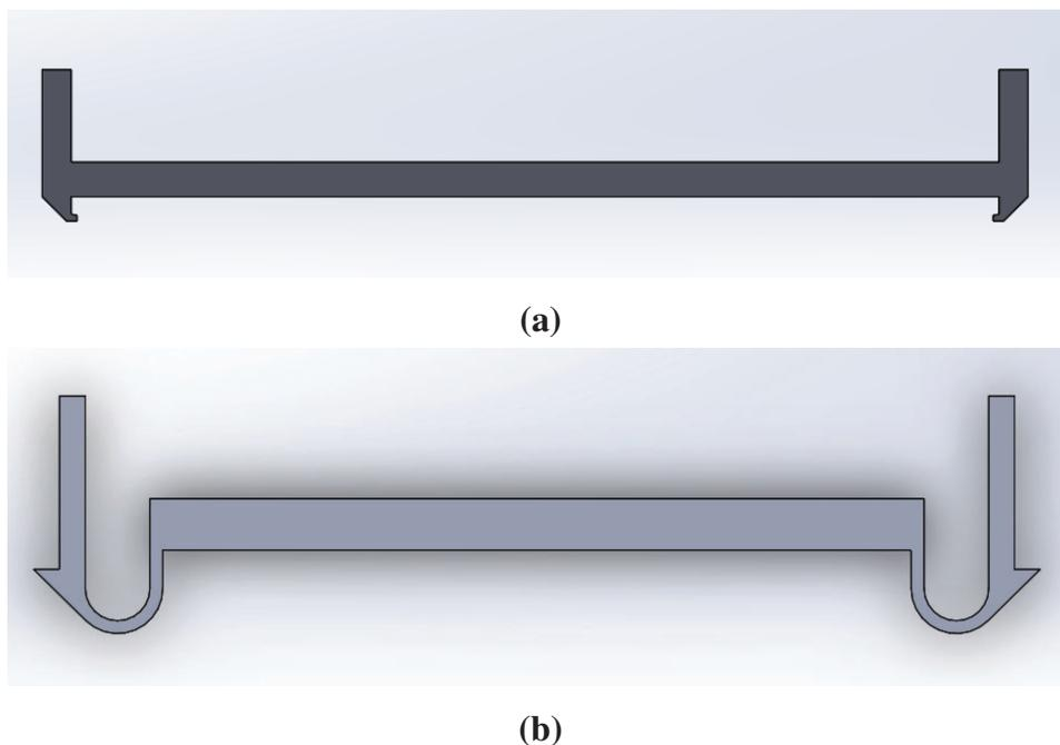
**Figure 5.9** The two connector prototypes, the one fastening on the outer edge (a) and the one fastening to the inner edge (b) of the metal grid of the motor end cap
