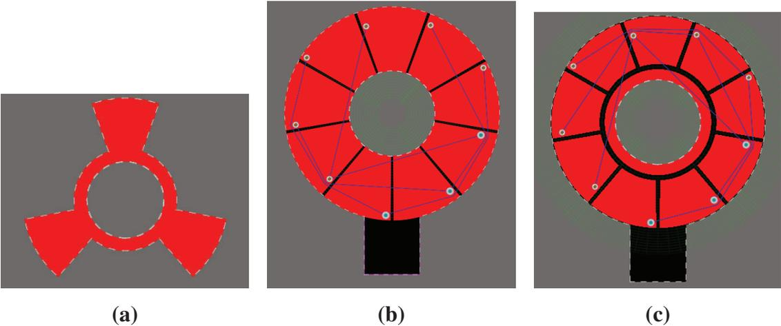
**Figure 5.4** PCB designs where the red areas are copper plated, the gray pins are connectors to the bottom layer and the blue lines are copper lines that connect pins. Seen in are the prototype designs of the rotor (a), the dual stator plate (b) and the single stator plate (c)
