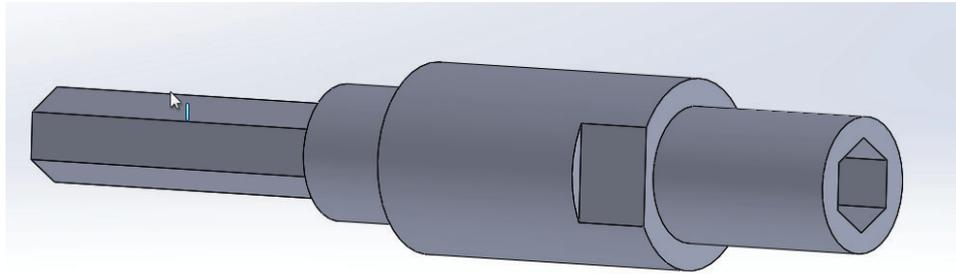
**Figure 5.7** CAD model of the final design of the shaft
