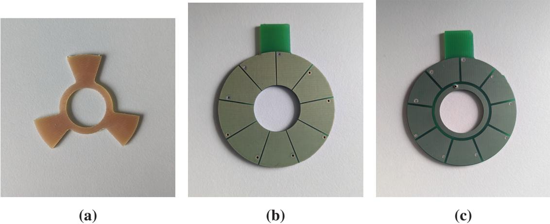
**Figure 5.5** Printed PCBs of capacitive encoder prototypes, seen are the rotor (a), the dual stator (b) and the single stator (c)
