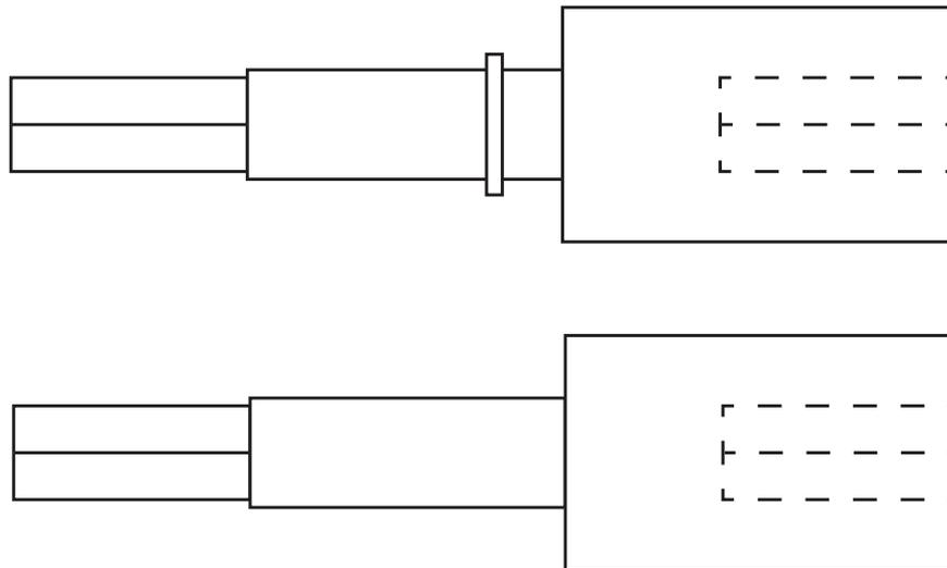
**Figure 4.1** Drawing of the shaft concepts, one with a lip for spacing of rotating encoder discs and one without.
