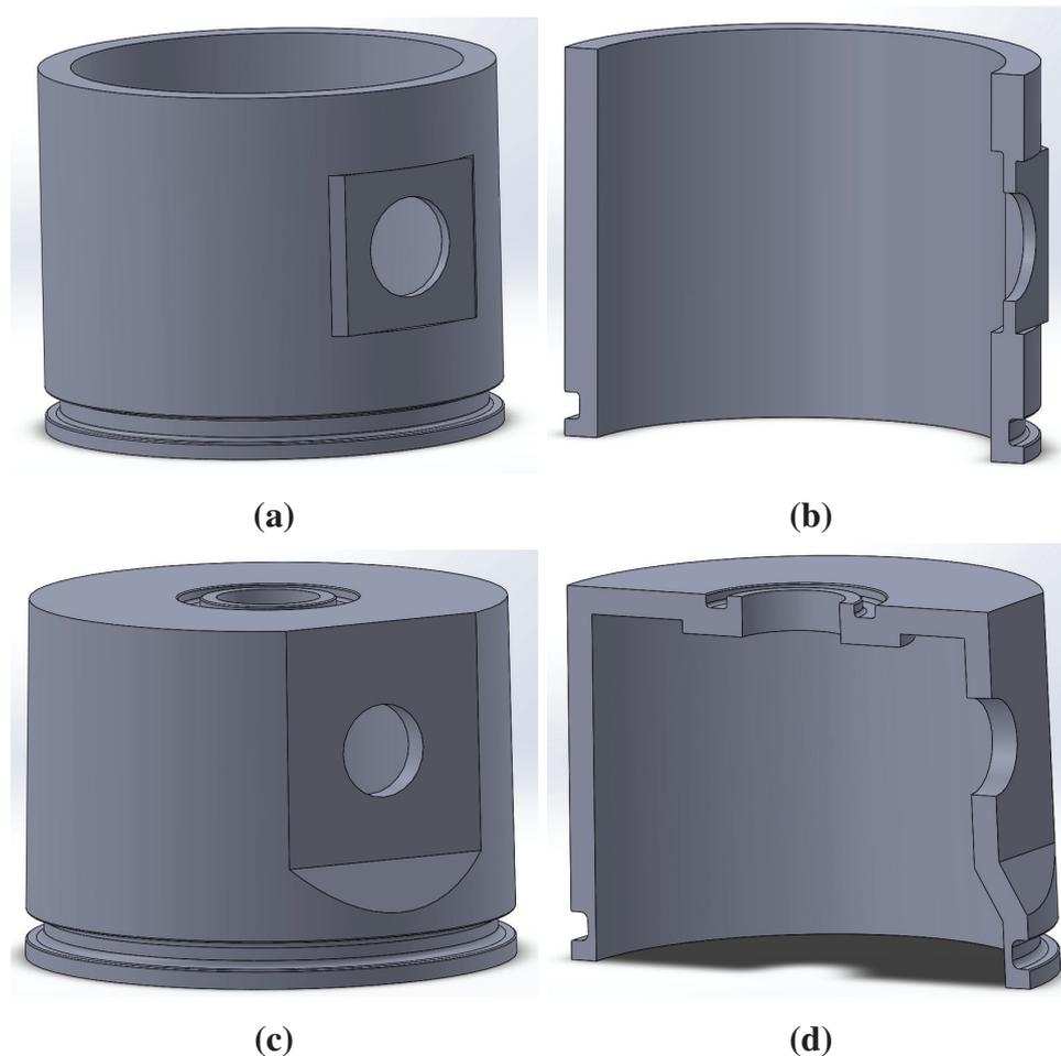
**Figure 5.13** The two housing prototypes, one with a flat area set into the cylinder (a) & (b) and one with a complete flat side (c) & (d), for connecting the cable gland along with cross-sections of them both
