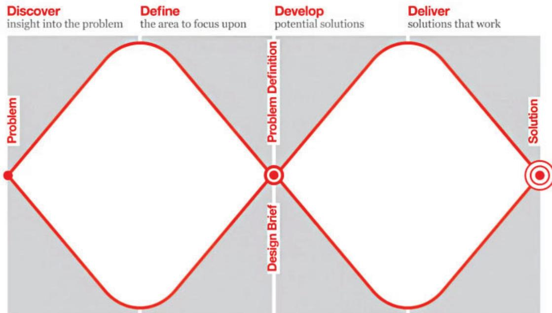
**Figure 3.2** An overview of the double diamond design process from [Costa, 2018]
