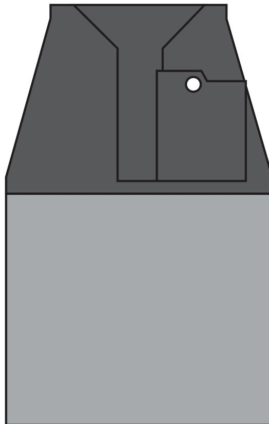
**Figure 5.15** A schematic assembly of the micro switch holder (dark grey) attached to the end of the encoder housing (light gray)
