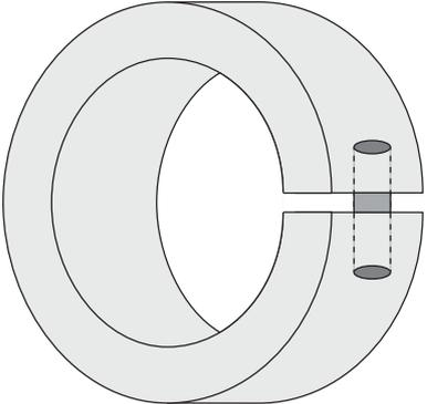
A 3D perspective drawing of a shaft collar. It consists of a single, thick, C-shaped ring with a central hole. A cylindrical shaft is shown passing through the hole, with a shaded section indicating the collar's contact with the shaft. The collar has a slightly tapered outer edge.                     | <p>Shaft collar - A readily available solution to clamp down on the motor shaft, may have difficulties properly clamping and centering a wide array of motor shaft diameters.</p> |
