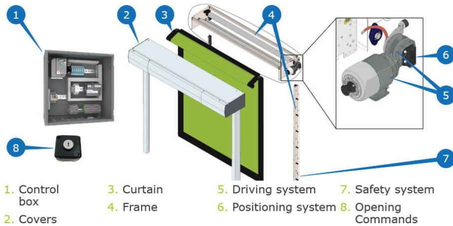
**Figure 1.1** Overview of high speed door system [Pede, 2021]
