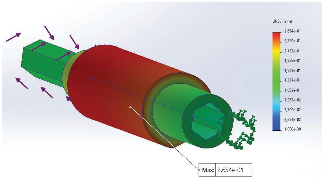
**Figure C.3** Simulated displacement results on the encoder shaft due to manual drive of the motor
